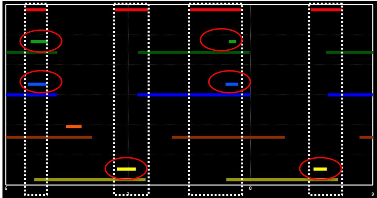
Green, Blue and Yellow: Times when satellite could be seen by offending earth station, where uplinking would occur
